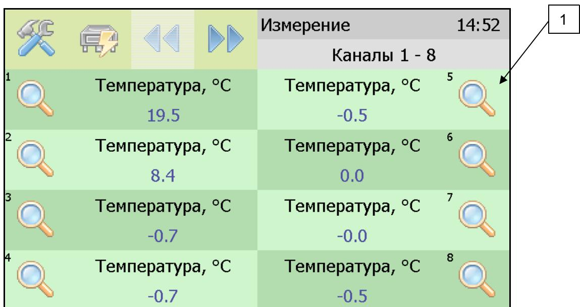
The screenshot shows a table with 8 rows, each representing a measurement channel. The columns are labeled: Измерение (Measurement), Каналы 1 - 8 (Channels 1 - 8), and time 14:52. Each row contains a magnifying glass icon, the parameter name, its unit ( $^{\circ}\text{C}$ ), and its current value. A callout box labeled '1' points to the top-left corner of the table area.
